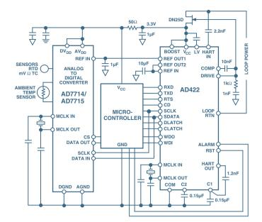
Figure 7. Complete intelligent transmitter with AD422
