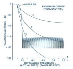
Figure 3. 90-tap FIR filter response compared with those of sharp cutoff Chebyshev filters.
