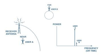
Figure 4. Near-far effect calls for the ability to handle wide dynamic range between adjacent channels.
