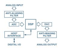
Figure 8. Putting together elements of a DSP system.
