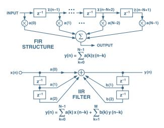
Figure 2. Filter equations and delay-line representation.
