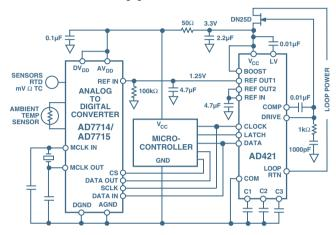
Figure 4. Details of a Smart Transmitter.
