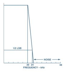
Figure 4. Antialiasing filter ideal response.
