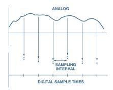
Figure 5. Sampling train and processing time.
